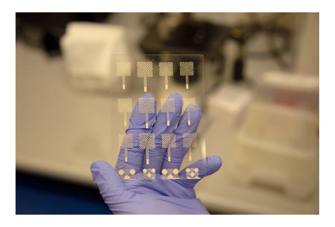
A set of screen-printed electrodes. Credit: Washington State University
