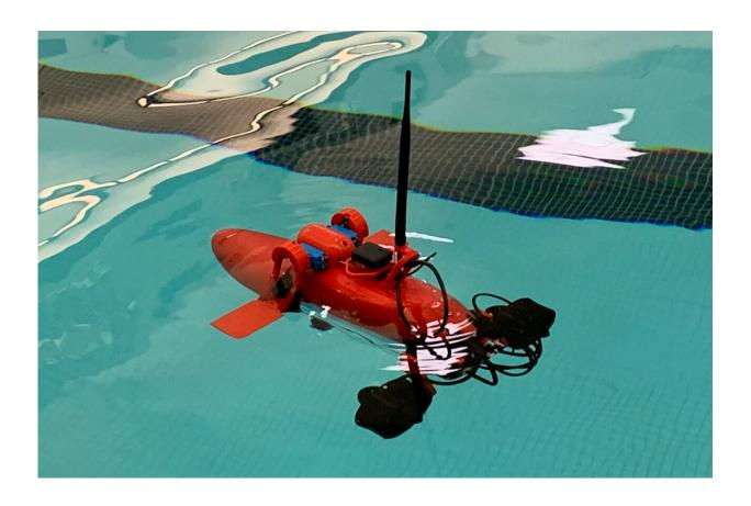
An unmanned semi-submersible vehicle prototype developed at Washington State University. Credit: Washington State University
