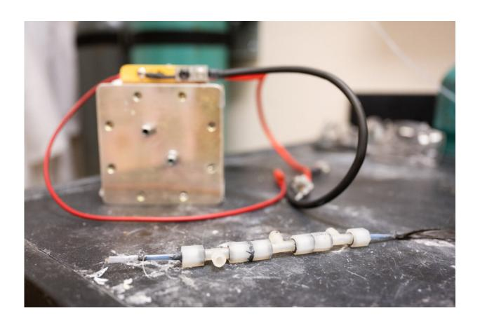
Liu's lab in the School of Chemical and Biomolecular Engineering (ChBE) developed a more compact flow battery cell configuration that reduces the size of the cell by 75%, and correspondingly reduces the size and cost of the entire flow battery. Credit: Georgia Institute of Technology
