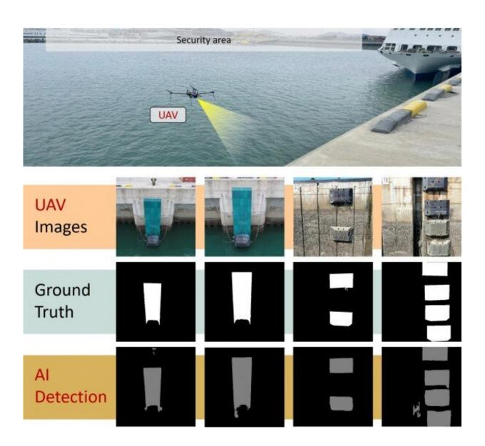
Port facilities in Incheon port, Korea, including fenders were captured by utilizing a UAV and then AI model detected only fenders in images with IoU and
