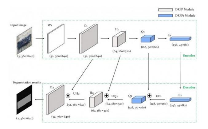
The encoder-decoder structure reduces and increases the size of the feature map using the stride convolution modules and pixel shuffle. Credit: Korea Institute of Civil Engineering and Building Technology
