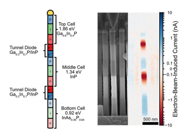
Nanowires in three materials imaged by a scanning electron microscope. A thread is a thousand times thinner than a strand of hair. The red and blue colour shows the direction of the current, and that the nanowires work as a tandem solar cell. Credit: Lund University
