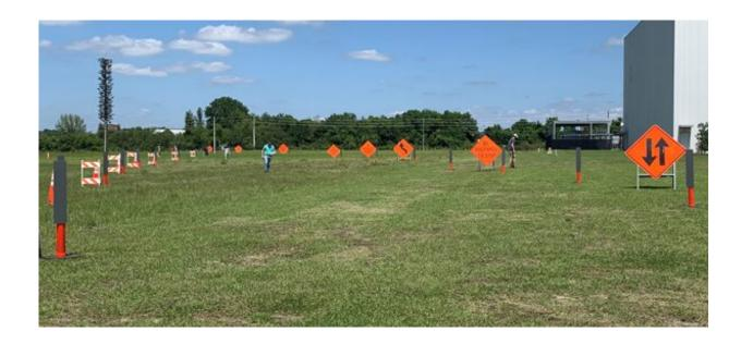
Reflective road signs were placed near the targets to measure the precision and range of automotive lidars under more challenging conditions. Credit: By the Authors, *Optical Engineering* (2023). DOI: 10.1117/1.OE.62.3.031211
