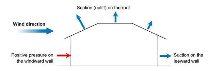
Typical external pressures on a sealed building. Credit: *Frontiers in Built Environment* (2022). DOI: 10.3389/fbuil.2022.970673
