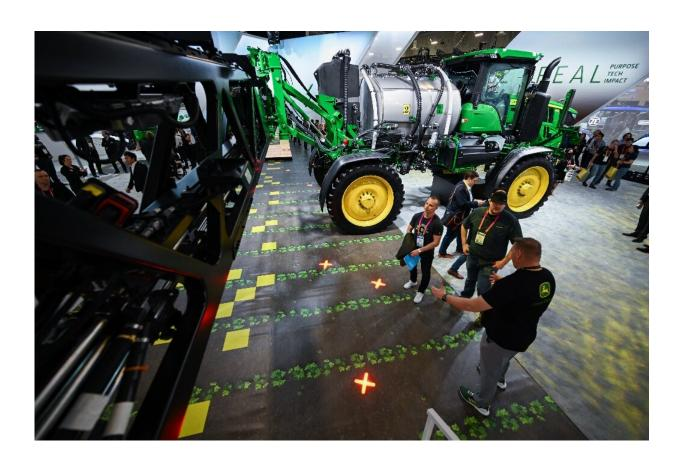
The new sprayers developed by agricultural giant John Deere, and displayed at the 2023 CES technology show in Las Vegas, Nevada, apply pesticides only where their cameras have detected weeds.
