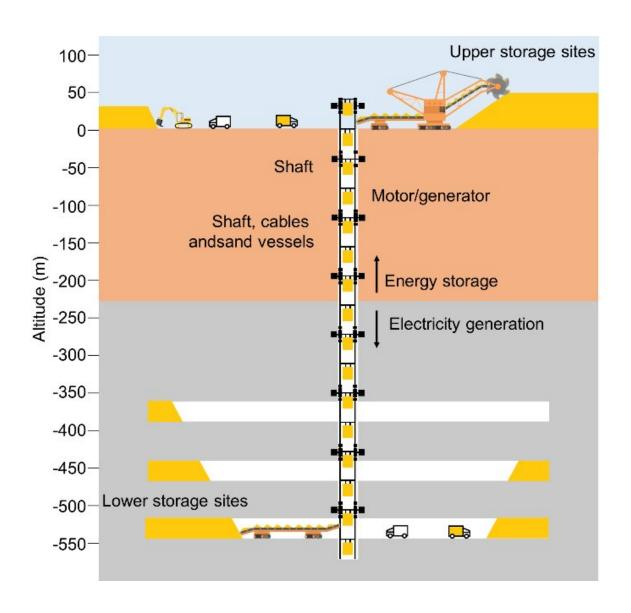
Underground Gravity Energy Storage system: a schematic of different system sections. Credit: Hunt et al.
