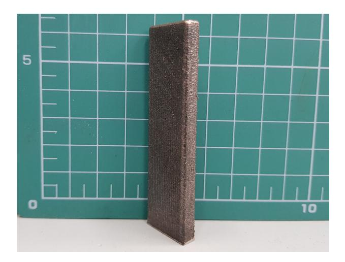
A vertical bar made of a quasi-homogeneous bronze-steel alloy manufactured by the researchers. Credit: Konstantin Makarenko/Skoltech.
