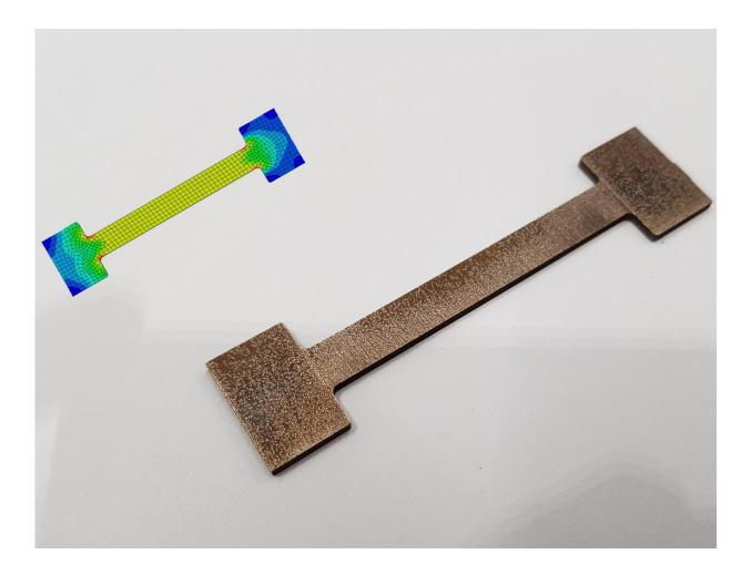
This is an example of a metal sample for mechanical tests. By subjecting it to stress, the researchers measure the material's strength, identify weak spots, such as the red spots on the stress map, and determine primary modes of failure. Credit: Konstantin Makarenko/Skoltech.
