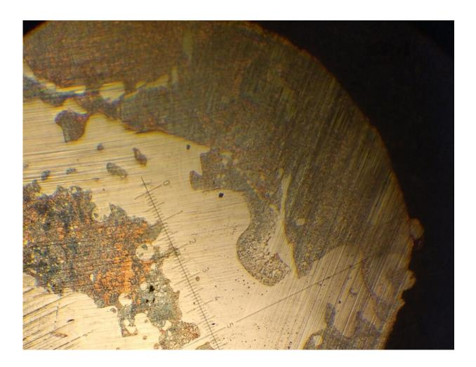
Alternating regions of bronze and steel in the bronze-steel alloy produced by the Skoltech researchers. The distance corresponding to one unit on the superimposed ruler is 0.1 millimeters. Credit: Konstantin Makarenko et al./Materials & Design.
