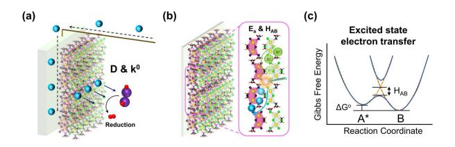
Schematic illustration of a photoelectrode deposited with a bismuth-based halide perovskite photocatalyst. (a) Heterogeneous electron-transfer kinetics during a photoelectrochemical hydrogen iodide splitting reaction. (b) Exciton transport dynamics of photogenerated electron-hole pairs; (c) Interfacial dynamics of excited state electron transfer. Credit: Dr Sam Hsu's research group/City University of Hong Kong
