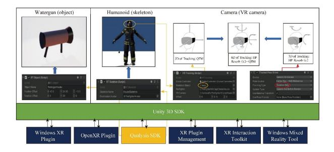
Figure shows the software components and synchronization of the VR environments of the training participants. Standard software development kits (SDKs,shown in dark blue in Figure) that help enable VR applications in Unity are available. Credit: Beijing Zhongke Journal Publising
