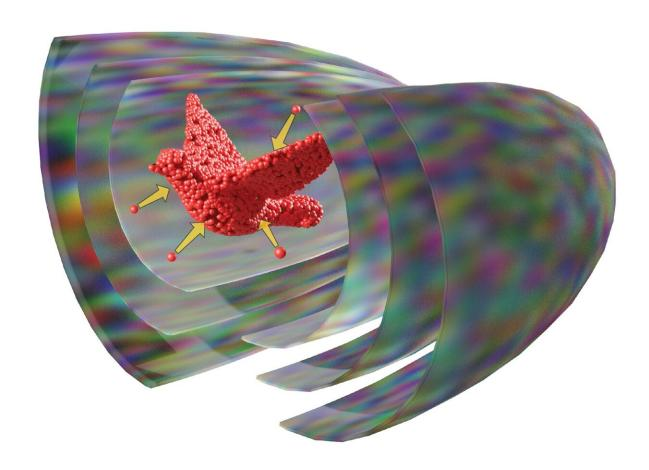
The use of sound waves to create a pressure field to print particles. Credit: Kai Melde, MPI für medizinische Forschung
