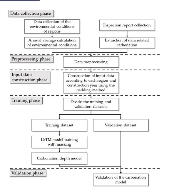
It shows the process from data collection related to carbonation to future prediction using artificial intelligence technique (LSTM) in the form of a detailed flowchart. Credit: Korea Institute of Civil Engineering and Building Technology
