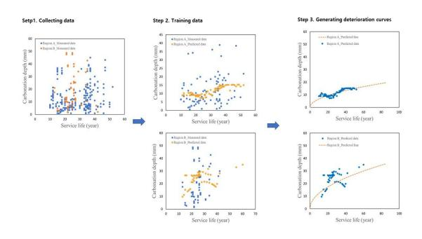
A process of setting the carbonation depth-related data collected in regions A and B as basic data and generating a future prediction curve for carbonation depth through a training process using artificial intelligence technology. Credit: Korea Institute of Civil Engineering and Building Technology
