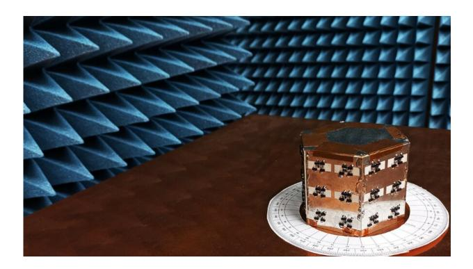
An international research team has developed reconfigurable antennas using artificially engineered structures called "metasurfaces" that can help solve the issue of limited frequency resources for wireless communications. These antennas provide variable response to waves of the same frequency but different pulse width. Thus, it provides a new degree of freedom to these antennas, making for more efficient data transfer. Credit: Hiroki Wakatsuchi from NITech, Japan
