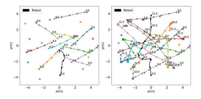
A colliding trajectory of a robot that has been trained using a standard exploration strategy (left) and a successful trajectory of a robot that has been trained with intrinsic rewards in the same scenarios. Credit: Martinez-Baselga, Riazuelo & Montano
