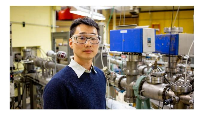
Part transmission electron microscope, part ion beam accelerator, Argonne's IVEM is one of about a dozen instruments in the world that lets researchers study material changes caused by ion irradiation as they happen. Chen conducts and facilitates user experiments at the facility. Credit: Seth Hoffman/Argonne National Laboratory.
