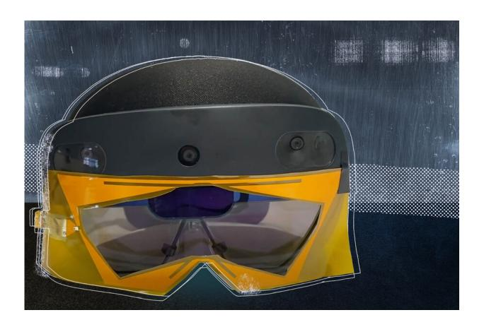
An augmented reality headset combines computer vision and wireless perception to automatically locate a specific item that is hidden from view, perhaps inside a box or under a pile, and then guide the user to retrieve it. Credit: MIT News
