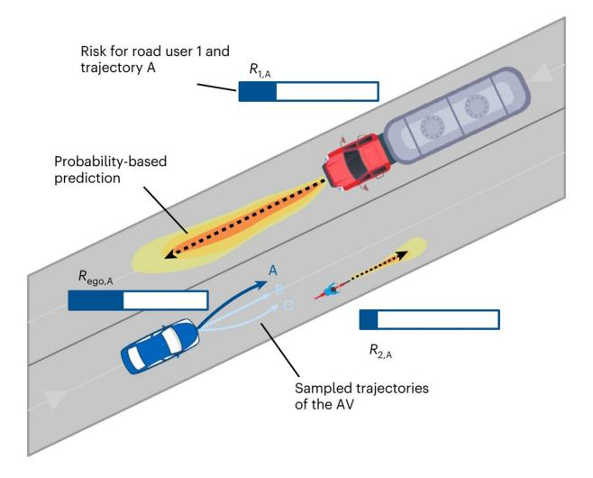
Trajectory planning based on risk distribution. On the basis of a probabilitybased prediction of all road users (shown here as heatmaps around the black most likely predictions) and an estimated harm value, every trajectory of the AV can be assigned risk values for every road user. Credit: *Nature Machine*
