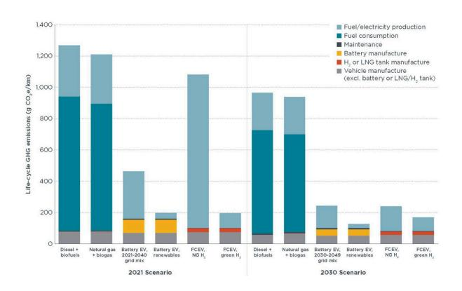
The comparison of the different powertrains and fuel options reveals that battery electric trucks take the lead in reducing life-cycle GHG emissions. Credit: © International Council on Clean Transportation.
