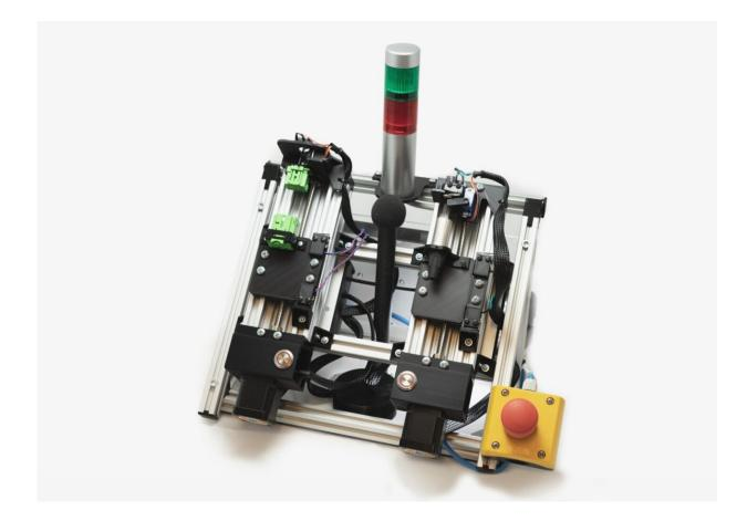
This demo device for click detection illustrates the reliable engagement of plug connections. The industrial traffic light indicates incorrect or correct engagement. Credit: Fraunhofer IDMT / Hannes Kalter
