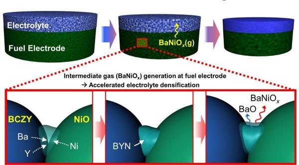
**Protonic Ceramic Cell Manufacturing Process**
