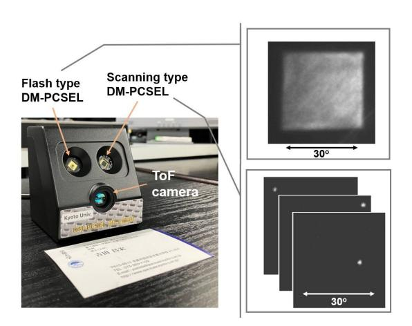
Researchers developed a new nonmechanical 3D lidar system, which is the size of a business card (seen in front of the system on the left). The system uses dually modulated surface-emitting photonic-crystal lasers (DM-PCSELs) as flash and beam-scanning sources. Credit: Susumu Noda, Kyoto University
