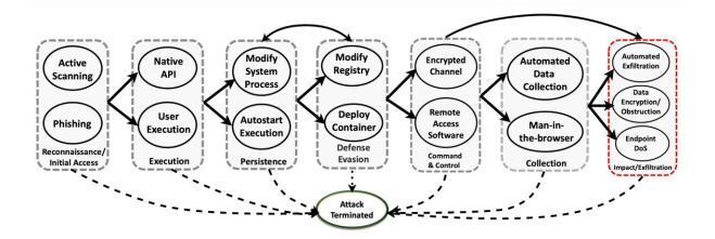
Multi-stage attack propagation represented with MITRE ATT&CK Tactics and Techniques. (Note: A directed edge between an attack tactic and technique specifies that the attacker may try to implement that technique next after achieving the objective of the attack tactic. Bidirectional arrow represents that Defense Evasion can come before Persistence.). Credit: *arXiv* (2023). DOI: 10.48550/arxiv.2302.01595
