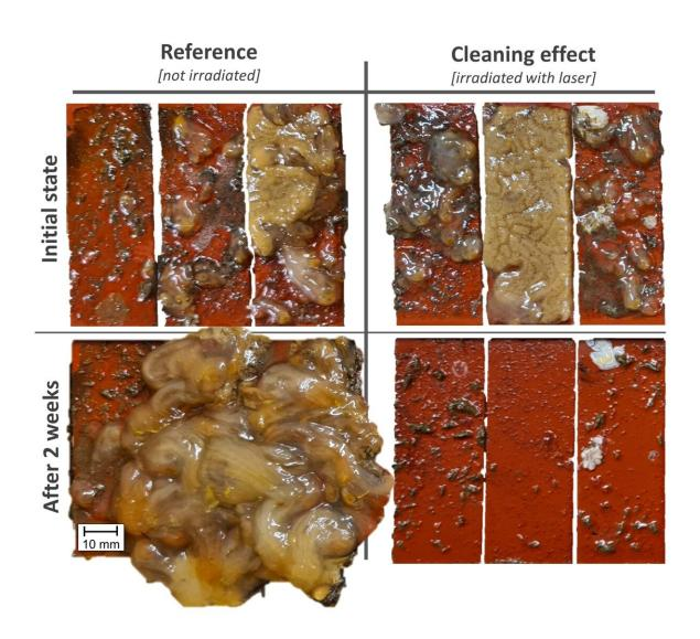
Results of the samples irradiated with the laser and those not irradiated. Credit: LZH
