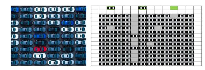
Left: Illustration of the density level of the envisioned automated garage system. Right: The grid-based abstraction with three I/O ports for vehicle dropoff and retrieval. Credit: Guo and Yu
