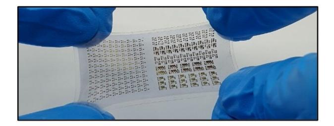
Image of intrinsically stretchable transistors and logic gates using a vacuum-deposited polymer dielectric. Credit: Prof. Donghee Son and Dr. Ja Hoon Koo.
