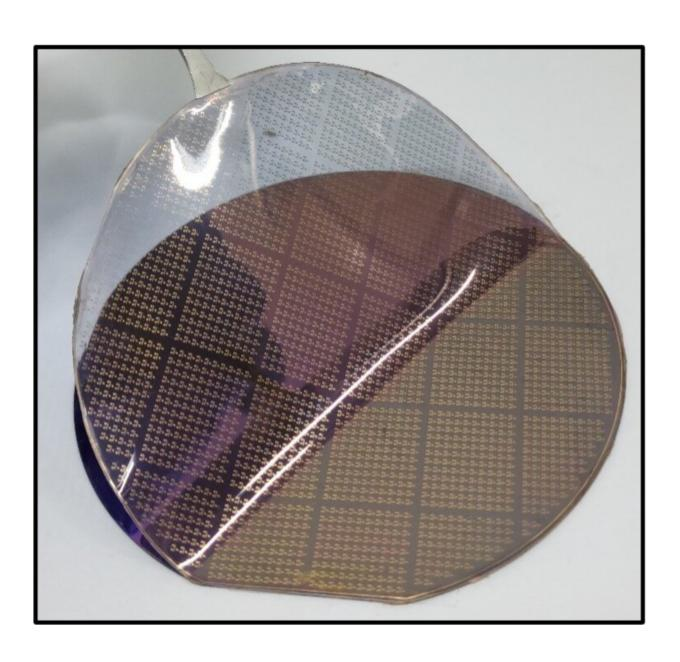
Photograph of wafer-scale fabrication of intrinsically stretchable transistor
