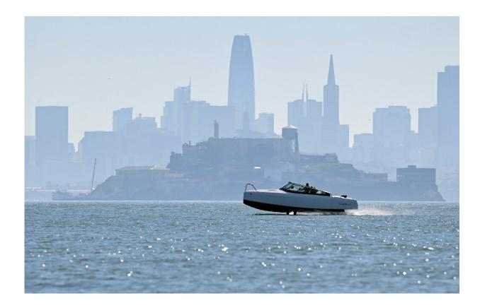
The hydrofoil technology lifts the boat out of the water during operations allowing for maximum efficiency at long range.
