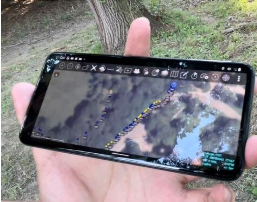
Screenshot of the "Cold Trailing" demonstration where the temperature data was registered with the GPS coordinates streamed from the firefighter's helmet in real-time. Credit: National Institute of Standards and Technology
