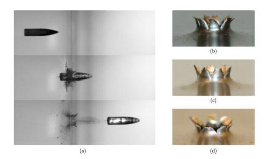
Image sequence of projectiles being fired through three different steel plates. The pictures on the right show the exit holes in the various plates. Credit: SFI
