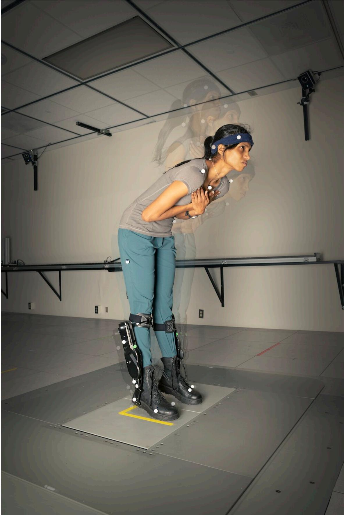
In this composite time series image, a test subject wearing a robotic lower-limb exoskeleton pitches forward but doesn't need to step to maintain her balance.
