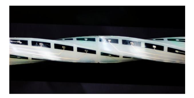
Sections of the team's flexible e-skin fitted to a soft robot arm. Credit: Yunjie Yang
