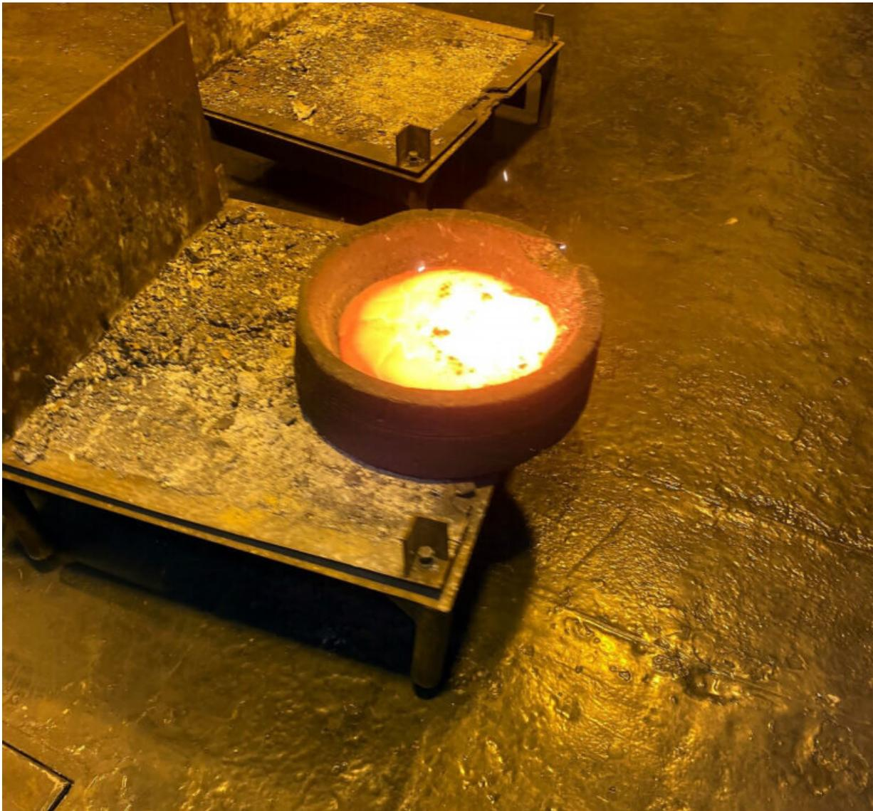
Finished silicon using the SisAl process. Credit: Norwegian University of
