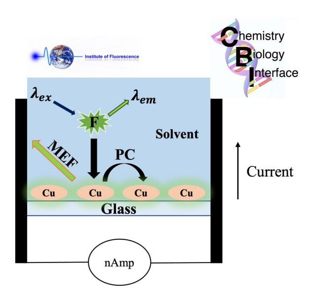
Plasmon to Current technology. Fluorophores produce an induced current in the metal, which is proportional to the magnitude of the fluorophore's extinction
