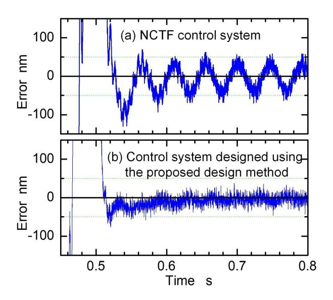
(a) Error of conventional NCTF control system(b) Error of proposed control system. Credit: *Precision Engineering* (2022). DOI: 10.1016/j.precisioneng.2022.11.008
