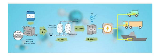
Fig. 2 Ammonia is split into nitrogen and hydrogen in the AMMONPAKTOR reactor. Hydrogen is converted in the fuel cells to produce power. Only a small amount of nitric oxide is produced thanks to the unique process design. Credit: Fraunhofer-Gesellschaft
