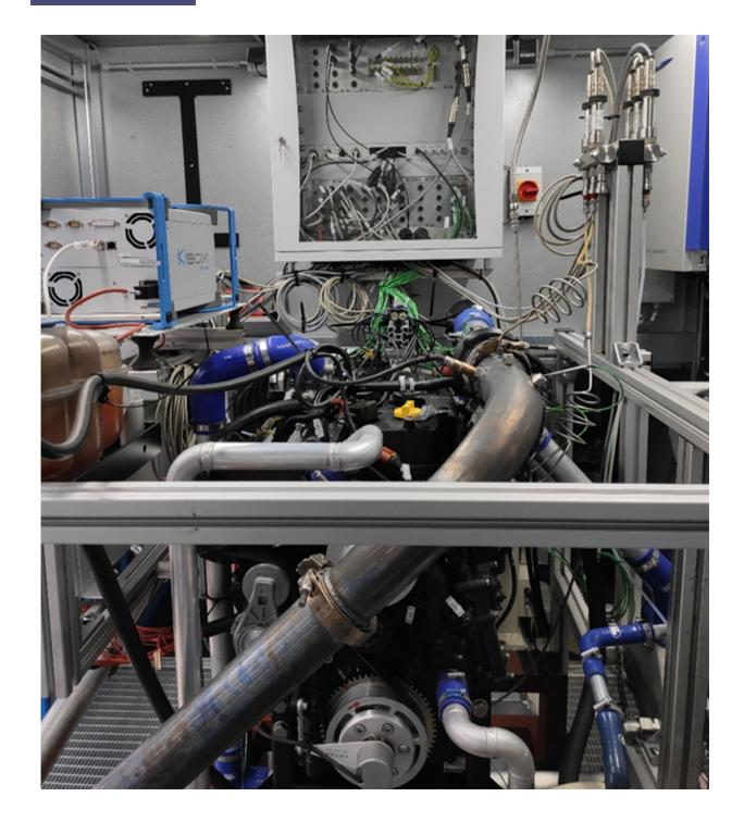
The concept was realized as a prototype. Extensive series of tests were completed on the injection nozzle test bench and on the engine test bench. Credit: Karsten Wittek, HS Heilbronn
