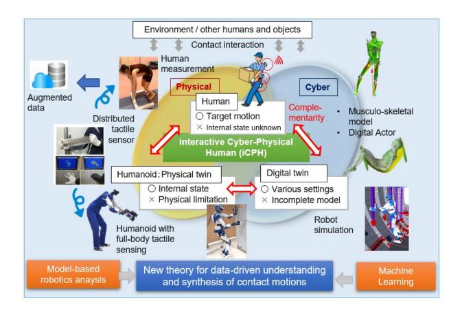
iCPH utilizes human measurement data, musculoskeletal analysis, and machine learning, enabling complementary humanoid robots (physical twins) and robot simulations (digital twins) to understand, predict, and synthesize human-like contact motions. Credit: Eiichi Yoshida from the Tokyo University of Science
