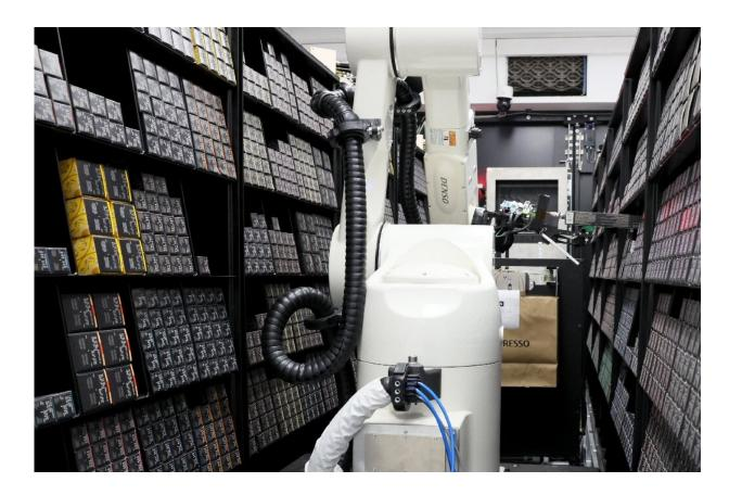
The robot receives the orders, packs and prepares them, with humans only needed to restock the warehouse and dispatch deliveries.
