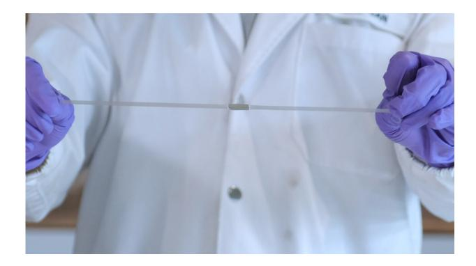
When subjected to stretching tests, modules were able to withstand stretching of up to seven times their original length before breaking. Credit: NTU Singapore
