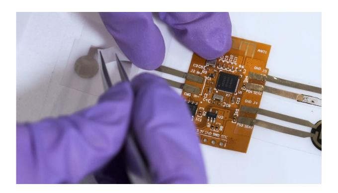
The BIND interface (biphasic, nano-dispersed interface) makes assembly of stretchable devices simple while offering excellent mechanical and electrical performance. Credit: NTU Singapore
