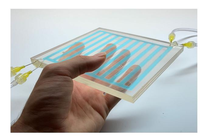
Prototypes of a multilayered fluidic system designed by U of T Engineering researchers contain several layers of channels that contain fluids with various optical properties. Credit: Raphael Kay, Adrian So
