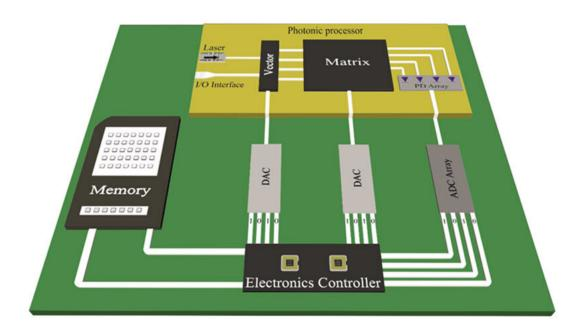
Electro-optic blocks cointegrated for the development of a neuromorphic photonic processor. Credit: Giamougiannis et al., doi 10.1117/1.AP.5.1.016004
