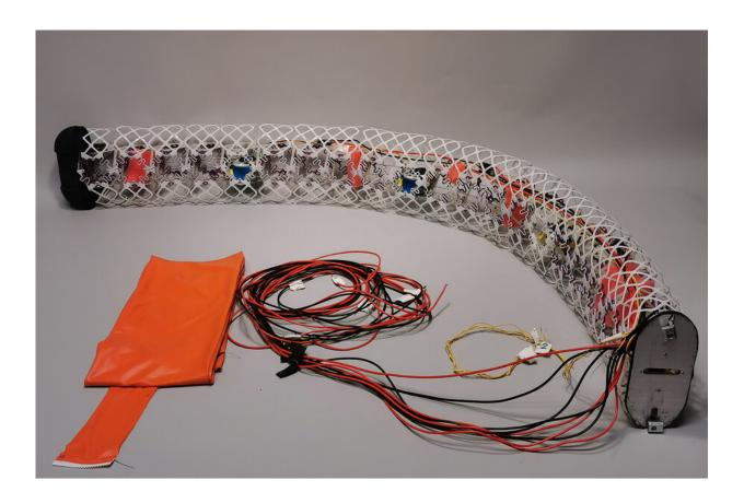
The deformable robots are made with lattice-like pieces, called voxels, that are low density and have high stiffness. Credit: Massachusetts Institute of Technology
