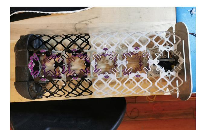
The individual voxels are mostly hollow structures made up of cast plastic pieces with narrow struts in complex shapes. Credit: Massachusetts Institute of Technology
