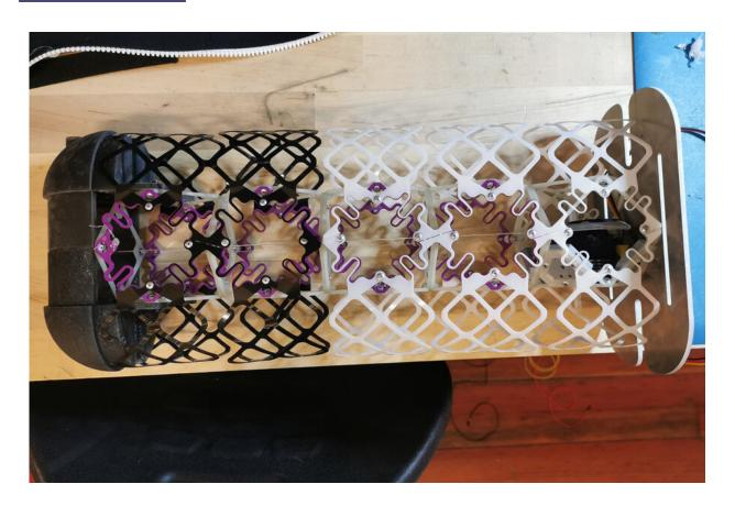
The individual voxels are mostly hollow structures made up of cast plastic pieces with narrow struts in complex shapes. Credit: Massachusetts Institute of Technology
