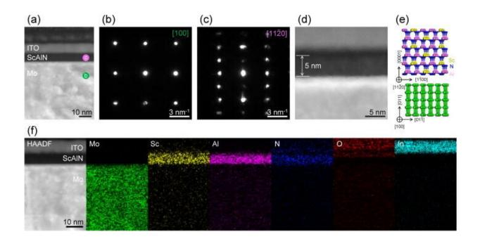
(a) Cross-sectional HAADF-STEM image of the 5 nm thick ScAlN grown on Mo template. (b) and (c) Nano-beam electron diffraction patterns captured from the Mo (b) and ScAlN (c) regions labeled in (a). (d) Magnified HAADF-STEM image showing the thickness of the ScAlN layer. (e) Schematic of the epitaxial relationship between wz-ScAlN and bcc-Mo. (f) EDS element maps for the ITO/ScAlN/Mo capacitor. Credit: *Applied Physics Letters* (2023). DOI: 10.1063/5.0136265
