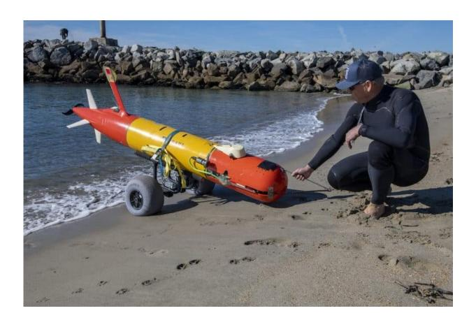
Mechanical engineer Brett Hobson—principal investigator and project manager for MBARI's Long-Range AUV team—inspects a Tethys-class LRAUV before launch from the beach adjacent to MBARI's research facilities. Credit: Tom O'Reilly © 2022 MBARI
