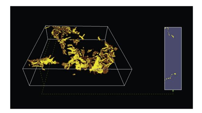
Molten salt corroded a metal barrier, appearing disconnected on a slice view of the damage (right). Researchers imaged the corrosion in multiple dimensions and reconstructed the path the salt took through metal (left). Credit: Yang Yang/Penn State
