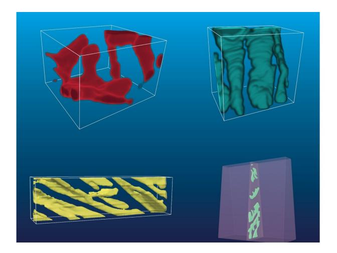
Molten salt penetrates various metal alloys in different patterns; oxide growth can form similar 1D morphology. From top left, clockwise: stainless steel corroded in salt, iron-nickel-chromium alloy corroded in salt, chromiummanganese-iron-cobalt-nickel alloy oxidized in air and nickel-aluminum alloy
