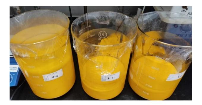
The recycled PbI<sub>2</sub> microcrystals exhibit the quality and purity levels necessary
