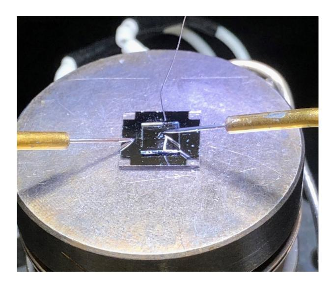
The pioneering solid-state electrochemical thermal transistor developed in this study. Credit: Hiromichi Ohta
