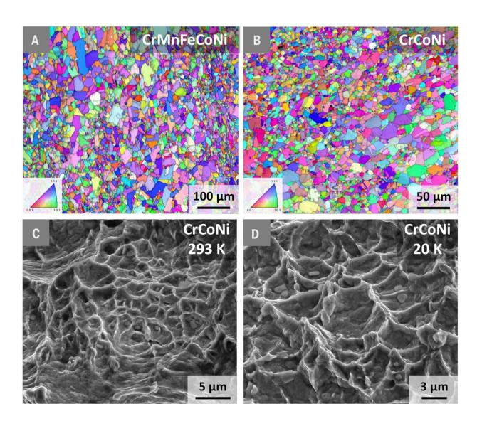
Microstructure and fractography of the CrCoNi-based alloys Credit: Dr Dong Liu
