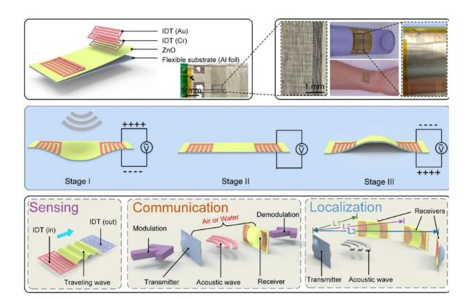
A graphic showing the principles of sensing and communication, acoustic ranging (identifying the distance), and positioning (finding locations) using the flexible acoustic wave device. Credit: Northumbria University
